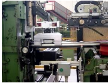
Inspection with bar rotation and translation by array probes
