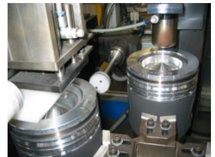
Inspection of hole and combustion chamber on a piston
