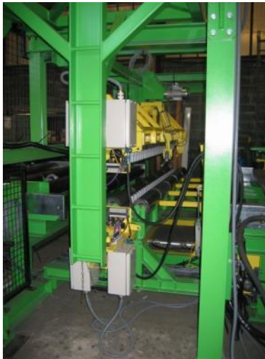
Inspection of electrical conductivity of aluminium alloys plates
